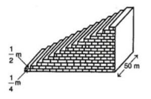
Each step has a rise of  $\frac{1}{4}$ m and a tread of  $\frac{1}{2}$ m (see figure). Calculate the total volume of concrete required to build the terrace.
